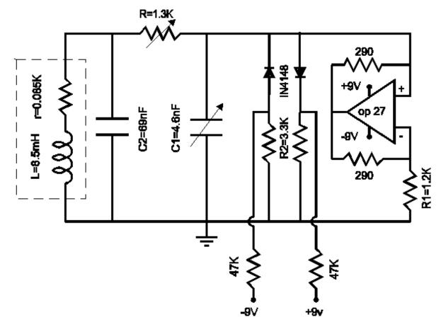
To see chaotic behavior, plot the voltage measured across C1 against the voltage measured across C2 (an X-Y oscilloscope with probes connected across these capacitors). The transition to chaotic dynamics can be found by *carefully* decreasing R or C1, (e.g. decrease R in steps of 0.01 to 1.2K). Source: http://www.cmp.caltech.edu/~mcc/chaos\_new/Chua.html
