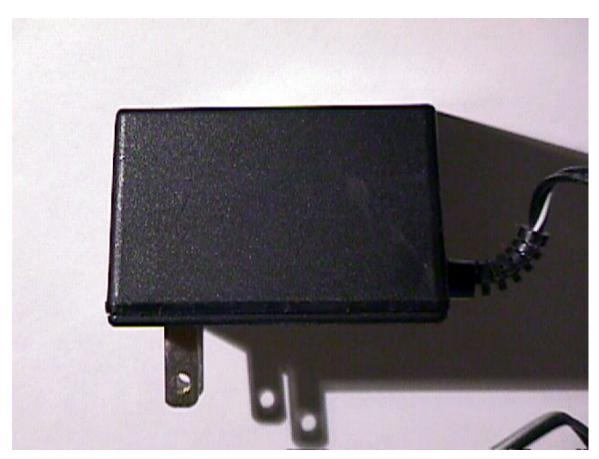
Old fashioned wall warts are linear power supplies, which are not very efficient. Newer ones are switching supplies (more efficient) – see below.
