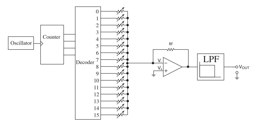
CMOS outputs (0 - 5 V) of decoder sum currents into an op-amp. By setting the pots to desired values, any 16-segment waveform can be synthesized.
